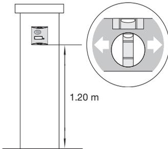
2. Mark and drill the outdoor caller unit holes with a  $\varnothing$  6 mm drill bit. Also mark the place where the cable feed hole has to be drilled ( $\varnothing$  8 mm min. recommended).
