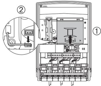
3. Remove the battery enclosure.
