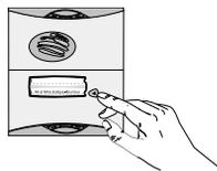
**IMPORTANT:** when using a translucent MHF01X or MHF02X outdoor caller unit and 1-button armoured cover, only the bottom key (KEY 1) can be accessed once the armoured cover has been placed on the unit.
