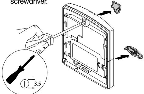
5. Thread the cable through the hole knocked out in step 3 and screw the caller unit in place. Put the screw covers back.
