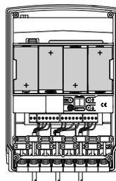
3. When the controller is powered, the radio link LED lights up red for 2 sec, the outdoor caller unit lights up and also beeps for 2 sec. If this is not the case, check the batteries have been correctly inserted.
