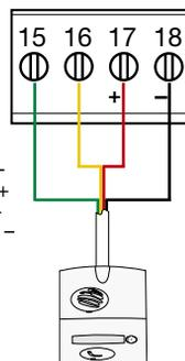
**TIP:** if the cable between the outdoor caller unit and the controller has to be extended, keep or shorten the length of the cable supplied and then connect the wires to a branch box in accordance with the rules below:
