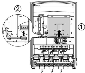
3. Remove the battery enclosure.
