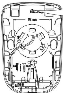
8. Rotate the back of the base until it is in wall position.
