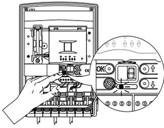
4. Press and hold
