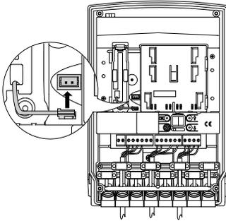
8. Connect a new MPU01X battery.
