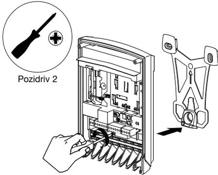
2. Following the installation rules below, mark 3 fixing points and drill a hole in the pillar using a  $\varnothing 6$  mm drill bit.
