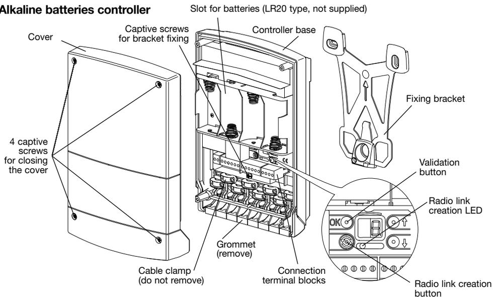
**IMPORTANT: the grommets, cable clamps and screws for the cable clamps are in the bag of accessories.**
