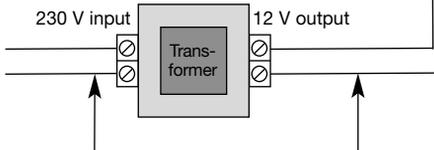
**IMPORTANT:** the transformer used must have the 12 V/10 VA min. double insulation symbol (230 V power supply without an earth connection).
