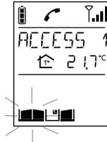
2. The gate at the access point making the call is activated within 5 seconds. At the end of communication, the gate status icon is updated (if a position contact is connected).
