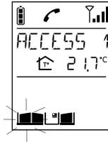
2. The side gate at the access point making the call is unlocked within 5 sec. At the end of communication, the side gate status icon is updated (if a position contact is connected).
