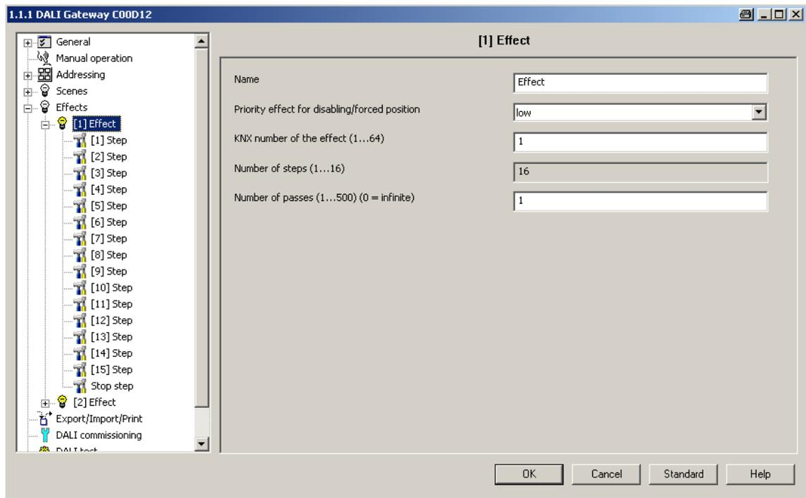
Figure 51: Configuration page of an effect as an example with 15 created effect steps and stop step
