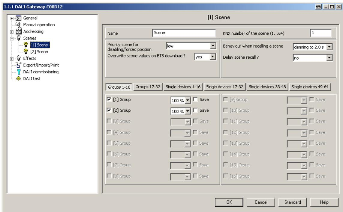
Figure 49: Configuration page of a scene as an example with two created effect scenes and two DALI groups
