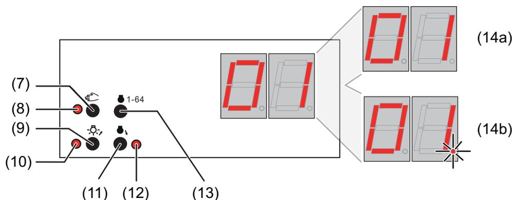
Figure 8: Controls and indicators for manual control
