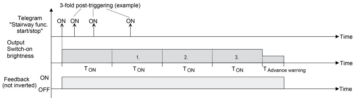
Figure 47: Time extension of the staircase function
