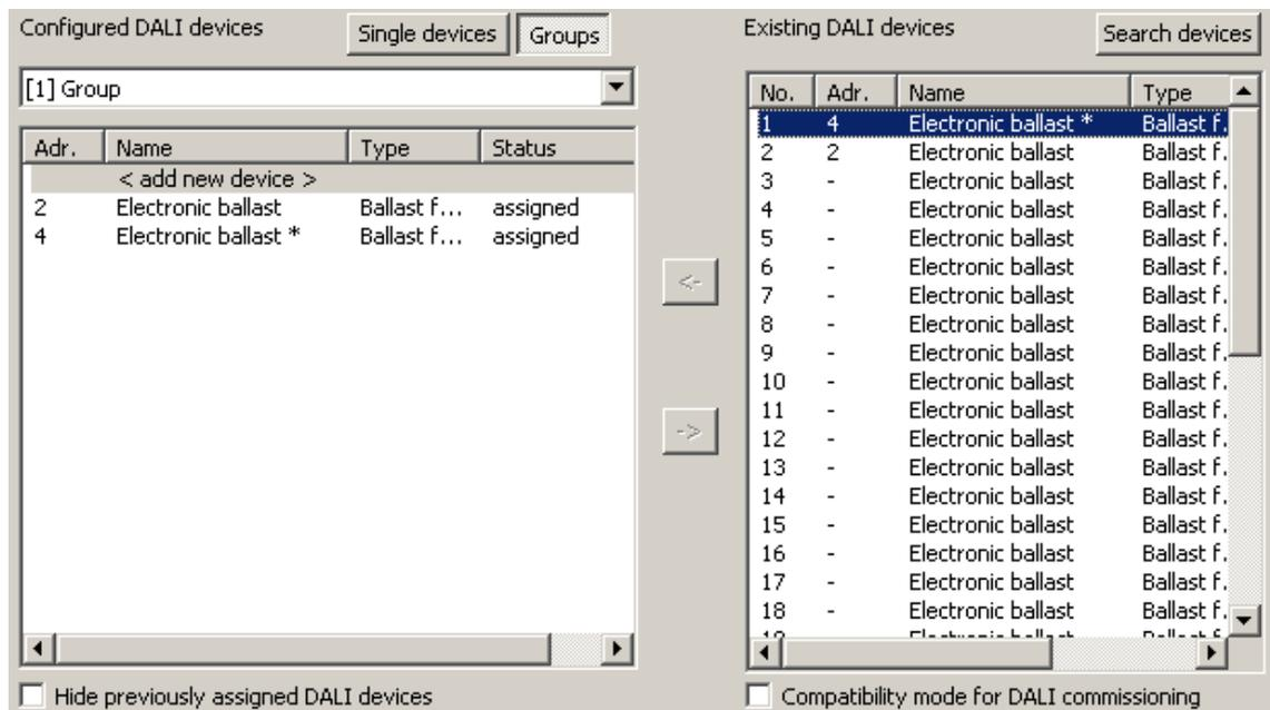
Figure 65: Operating device assigned to a group
