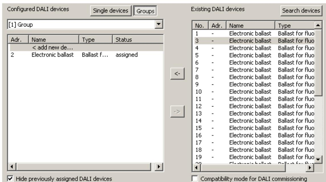
Figure 64: Operating device assigned to a group
