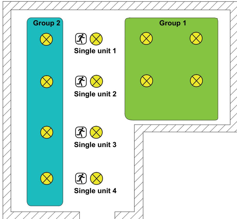
Figure 14: Example of group and single device control with single-battery-operated emergency lights
