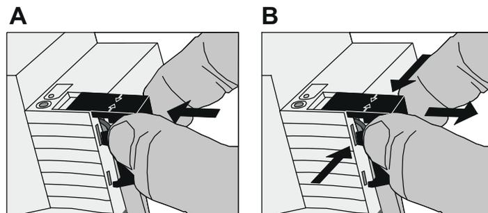
Figure 7: Installing / removing the protective cap
