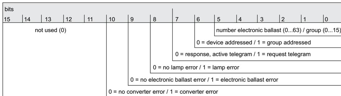
Figure 30: Telegram structure, 2-byte KNX error status
