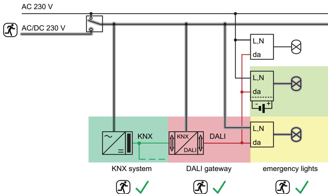
Figure 21: Example of a combined application of a centrally-supplied emergency lighting system with single-battery-operated DALI emergency lights
