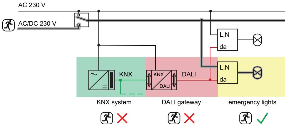
Figure 17: Example of a central supply - Only DALI operating devices integrated into the emergency power supply
