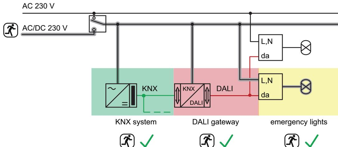
Figure 19: Example of a central supply - DALI operating devices, KNX system and DALI Gateway integrated into the emergency power supply
