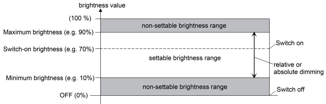
Figure 35: Settable brightness range when dimming (example)
