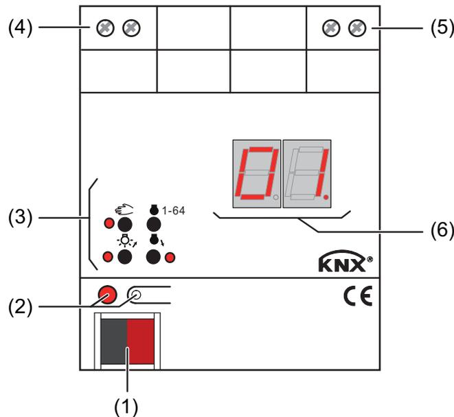
Figure 1: Device components
