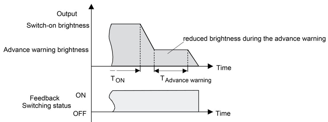
Figure 44: The pre-warning function of the staircase function with soft OFF function (as an example with minimum brightness = 0 %)
