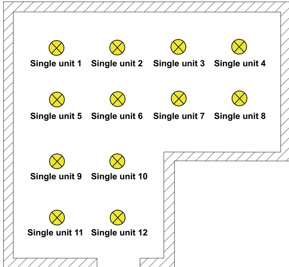
Figure 15: Example of single device control - All the DALI operating devices can be controlled individually
