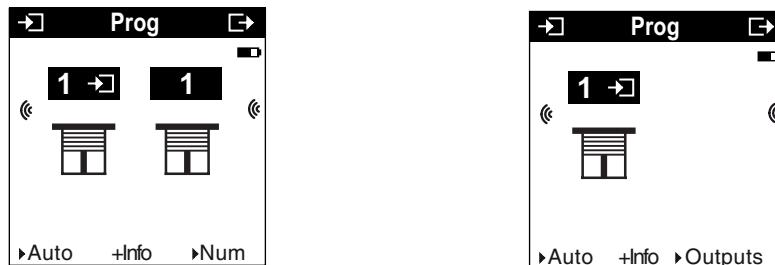
The +Info mode allows the status indication to be linked from an output to a viewing product: Area controller, LED output, etc. The status indication sends the current status over the network each time the status changes.
