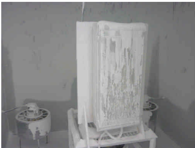
fig. 3 specimen in the dust chamber after the dust test (IP5X)
