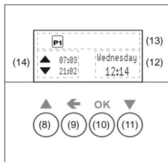
Figure 2: Display and operating elements
